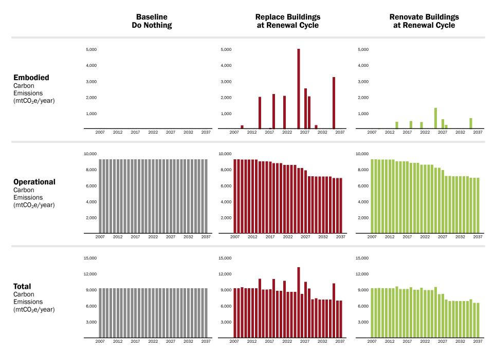
FIGURE 17 Each scenario to do nothing, replace buildings at renewal cycle, or renovate buildings at renewal cycle has unique implications on embodied and operational emissions over time.
